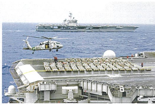
Cool side view from the Fantail of G-1 Flight Deck Crew with Hooking up pallets of BLU-110 to HSC-7 Dusty Dogs Helo with the USS Theodore Roosevelt CVN-71 in the back ground receiving her TOP OFF.
