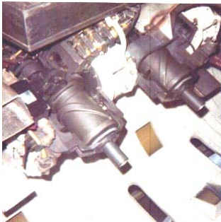
XM-149 40mm Honeywell grenade launchers in the forward bomb bay. - photo submitted by Rich Gadomski
