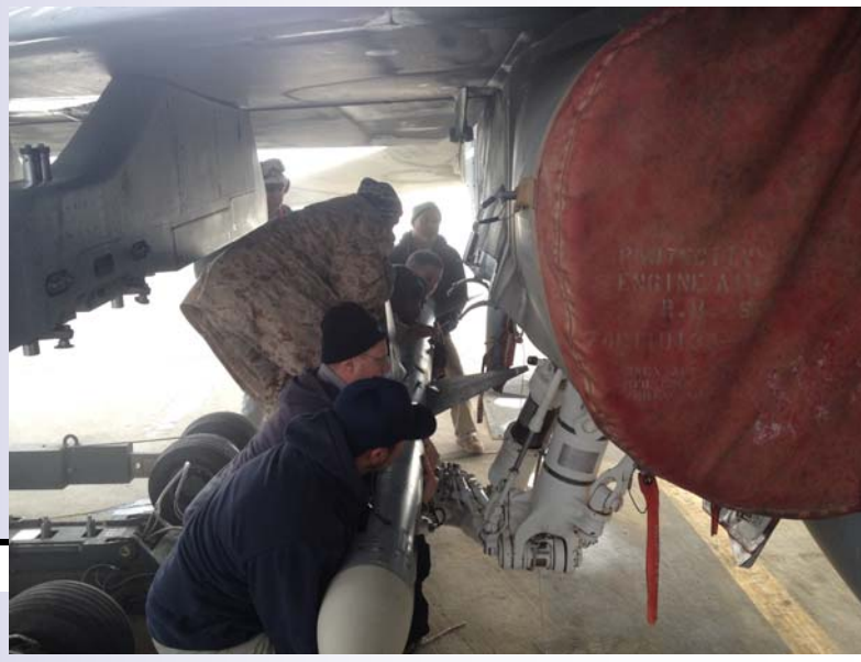
GBU-38 and AIM-120 training for the Kuwait Air Force along with Kay & Associates INC Ordnancemen .....Notice the MK 43 TDD, they still use the good ole M904E4
